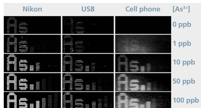
Microfluidic encapsulation-enabled microbial sensor array for monitoring arsenic contamination, showing different output patterns on various arsenic (As<sup>3+</sup>) levels. Left, middle, right panels: images acquired by a Nikon microscope, USB fluorescence microscope and cell phone camera.
