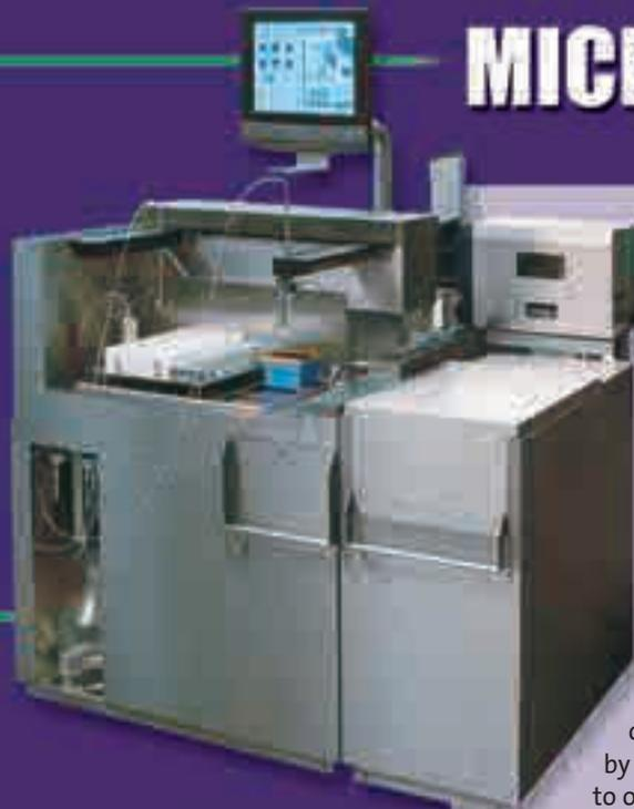
ROHASYS has developed a fully automatic diluting and sample dispensing system to carry out many of the processes on microbiological samples: the MICROBOT. With very high accuracy the samples (e.g. food, medical or environmental) are diluted and dispensed into petri dishes.
