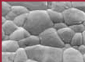
**Figure 2b.** A thin film of normal metallic silver sputtered by vapour deposition onto a surface. Modified from Dunn & Edwards-Jones (3)
