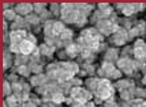
**Figure 2a.** A thin film of nanocrystalline silver sputtered by vapour deposition onto a surface
