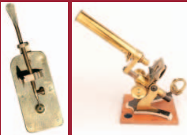
Figures 2 and 3. A representation of the first microscope (left) and a compound microscope (right)
